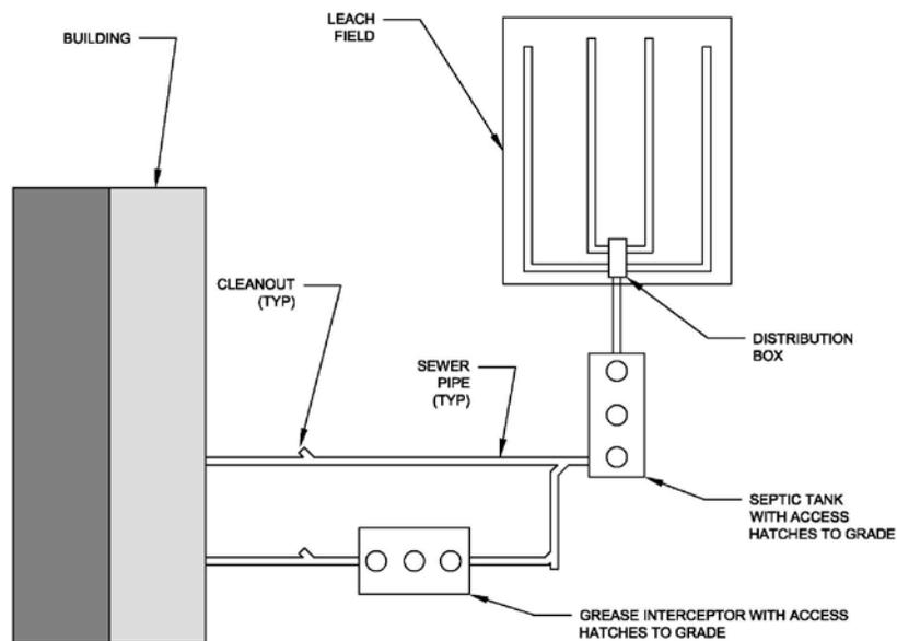
**Figure D-1 Type II Grease Interceptor and Septic Tank Building Sewers Discharging to Soil-Based Treatment Systems (STS)**
