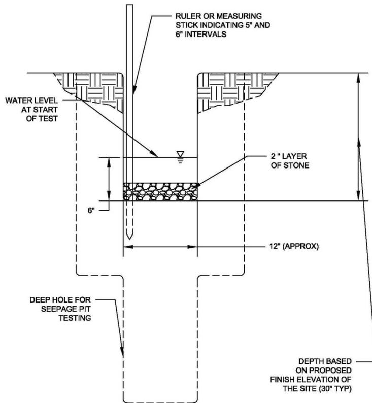
**Figure B-1 Soil Percolation Test Arrangement**
